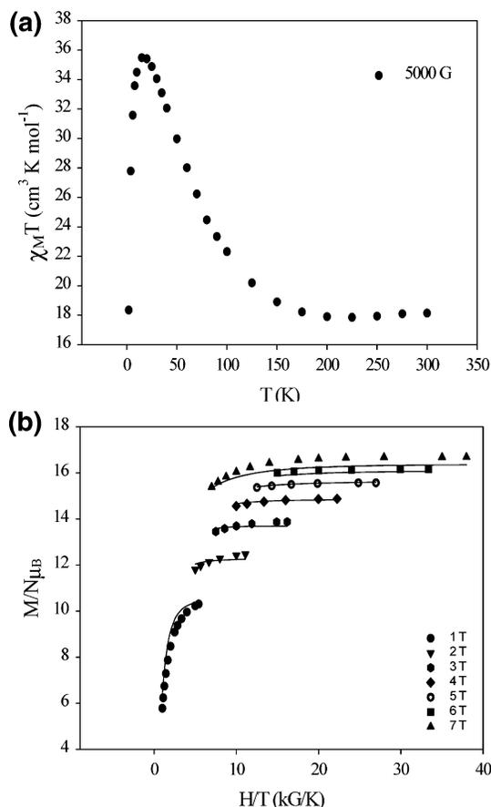
**Figure 2.** (a) Plot of  $\chi_M T$  versus  $T$  for complex **1** measured in the temperature range of 1.8–300 K in a field of 5.0 kG. (b) Plot of reduced magnetization ( $M/N\mu_B$ ) versus  $H/T$  for complex **1**. The solid lines are fits of the data to an  $S = 17/2$  state with  $g = 1.97(3)$  and  $D = -0.29 \text{ cm}^{-1}$ . Data were measured at 1–7 T and 1.8–4 K.
