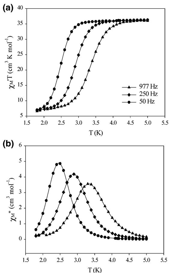
**Figure 3.** Plots of the in-phase ( $\chi_M'$ ) signal as  $\chi_M'T$  and out-of-phase ( $\chi_M''$ ) signal in ac susceptibility studies versus temperature in a 3.5 G field oscillating at the indicated frequencies.
