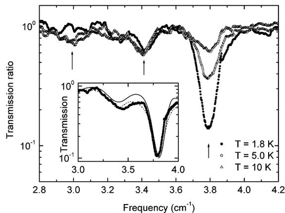
**Figure 6.** Normalized FDMRS spectra recorded on a pressed powder pellet of **1** at various temperatures, as indicated in the figure. The inset shows the 1.8 K non-normalized spectrum together with fits assuming Gaussian (solid line) and Lorentzian (dotted line) line shape functions.
